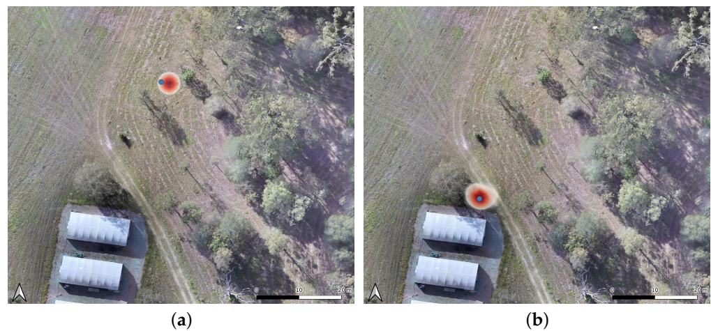
Figure 15. GNSS coordinates' heatmaps of confirmed victim detections by the POMDP-based motion planner in hybrid flight mode. (a) First victim location (blue dot) in an open area. (b) Second victim location (blue dot) nearby a tree.
