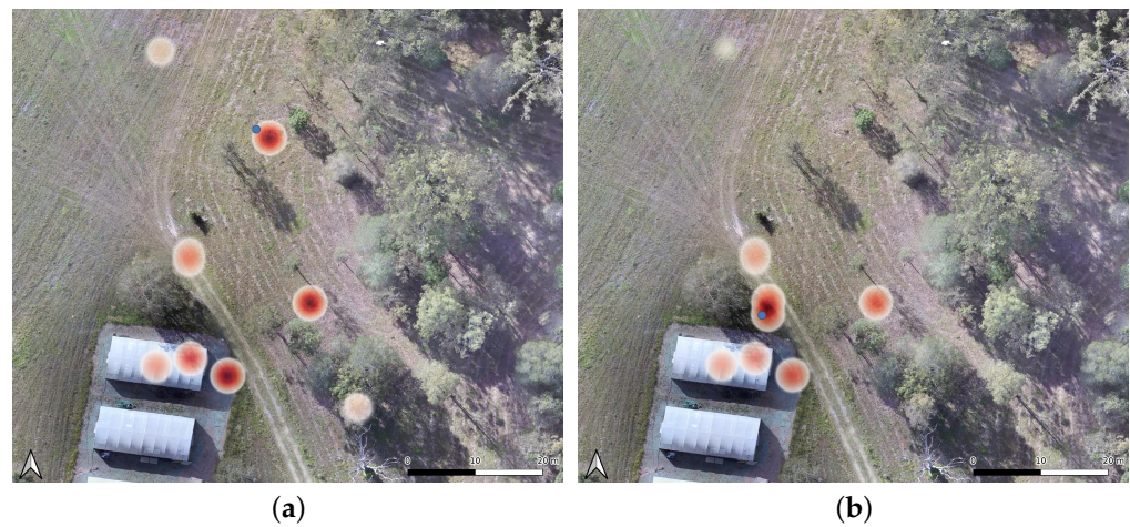
Figure 13. Heatmaps from recorded GNSS coordinate points from detections in mission mode. The amount of false positive locations were triggered by the CNN model from detecting other objects as people during the survey. (a) First victim location (blue dot) in an open area. (b) Second victim location (blue dot) nearby a tree.
