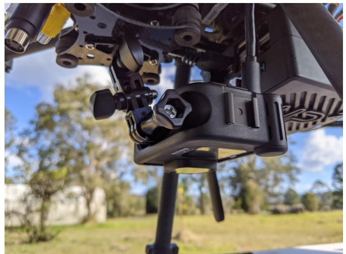
Fig. 4. GoPro Hero 9 mounted onto an anti-vibration bracket, pointing to the ground and in parallel to Earth's nadir.
