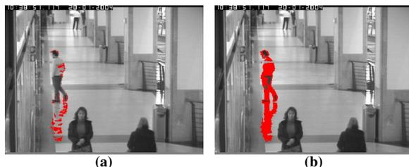
**Figure 1.** Detection rate and discrimination rate trade-off in chromacity based shadow detection (the original scene is shown in greyscale rather than in colour for ease of interpretation only). Red areas indicate pixels classified as being part of the person's shadow. Higher thresholds used in (a) reduce the shadow detection rate. Lower thresholds used in (b) increase the detection rate but reduce the discrimination rate.
