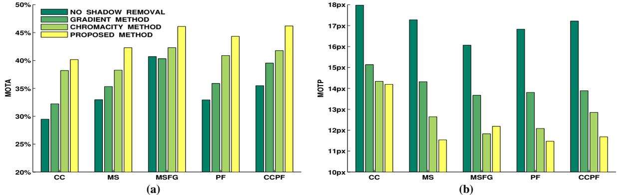
**Figure 3.** Effect of shadow removal methods on: (a) multiple object tracking accuracy (MOTA), where taller bars indicate better accuracy; (b) multiple object tracking precision (MOTP), where shorter bars indicate better precision. Results are grouped by tracking algorithm: blob matching (CC), two mean shift trackers (MS and MSFG), particle filter (PF) and hybrid tracking (CCPF).
