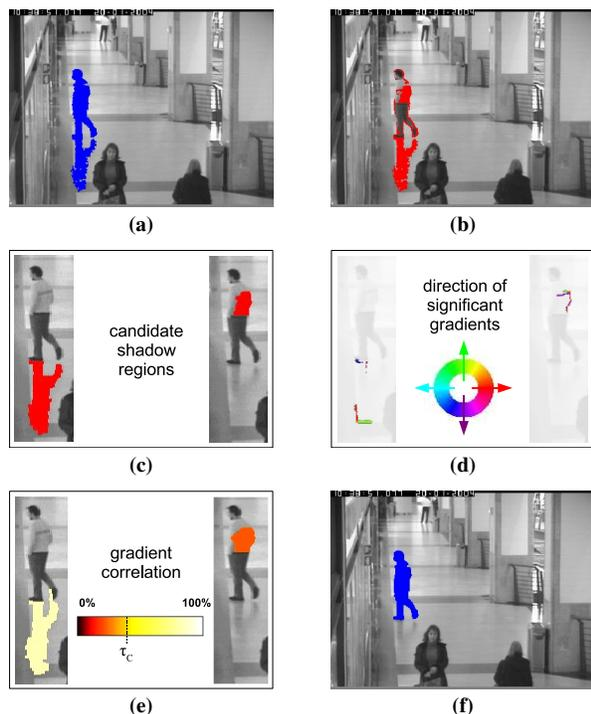
**Figure 2.** Processing in the proposed method: (a) foreground obtained after background subtraction, marked in blue; (b) pre-selection of shadow pixels based on chromacity; (c) candidate shadow regions; (d) gradient direction of pixels with significant gradient magnitude; (e) gradient direction correlation for each candidate region (only the region in the left pane is above the threshold  $\tau_c$ ); (f) final foreground object pixels marked in blue, omitting the shadow.
