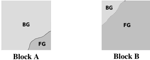
Figure 1. Misclassification is inevitable at the pixel level whenever a given block has both foreground (FG) and background (BG) pixels. Classifying Block A as background results in a few false negatives (foreground pixels classified as background) while classifying Block B as foreground results in a few false positives (background pixels classified as foreground).
